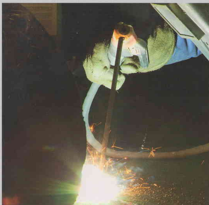
Production of VAUTID wear plates
