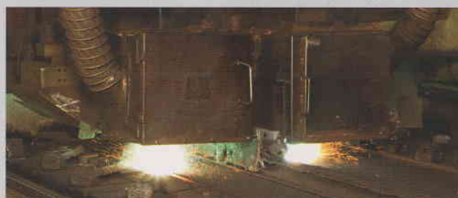
Production of VAUTID wear plates
